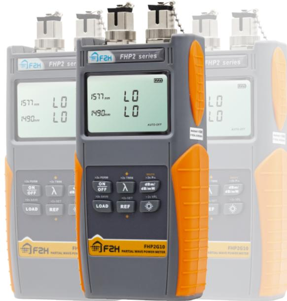
With the gradual upgrading of EPON/GPON network to 10G-EPON/XG(S) PON, the downstream of PON network will exist two wavelengths of 1490nm and 1577nm, which cannot be distinguished and measured separately by ordinary broadband power meter. FHP2G10 is a professional instrument specially used to measure the downstream 1490nm and 1577nm power levels of 10G-EPON/XG(S) PON network. It can accurately measure the optical power value of each wavelength and display it on one screen at the same time.
